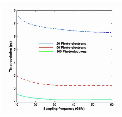
Simulated timing resolution vs Sampling rate 50PEs (white + detector noises)
