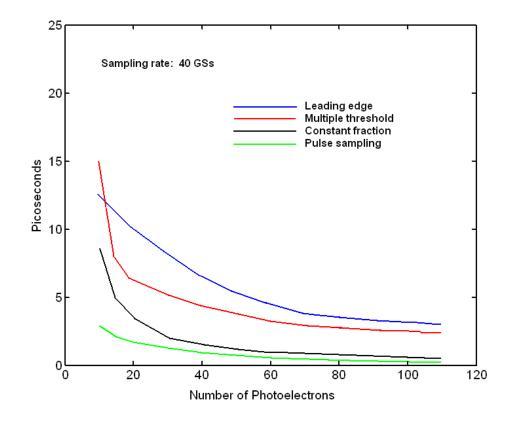
Simulated timing resolution using fast sampling S/N=80 at 50PEs (white + detector noises)
