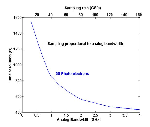
Simulated timing resolution vs Sampling rate and analog bandwidth 50PEs (white + detector noises)
