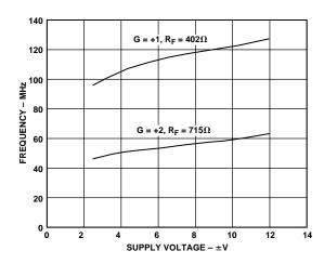
TPC 6. Bandwidth vs. Supply,  $R_L = 500 \Omega$ ,  $V_{IN} = 200 \text{ mV} p-p$
