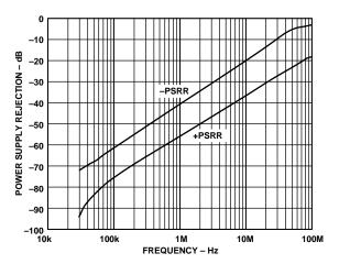
TPC 30. Power Supply Rejection vs. Frequency,  $V_S = \pm 12 V$
