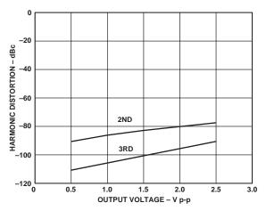
TPC 19. Distortion vs. Output Voltage,  $V_S$  = ±2.5 V, G = +1, f = 1 MHz,  $R_L$  = 500  $\Omega$ ,  $R_F$  = 0  $\Omega$
