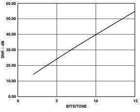
Figure 4. ADSL DMT SNR vs. Bits/Tone
