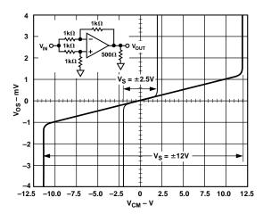
TPC 27. Voltage Offset vs. Input Common-Mode Voltage
