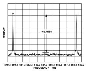
TPC 23. Multitone Power Ratio:  $V_S = \pm 6 V$ ,  $R_L = 500 \Omega$ , Full Rate ADSL (DMT), Downstream
