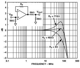
TPC 1. Frequency Response vs.  $R_F$ , G = +1,  $V_S = \pm 12$  V,  $V_{IN} = 63$  mV p-p
