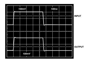
TPC 10. Noninverting Small Signal Pulse Response,  $R_L = 500 \ \Omega$ ,  $V_S = \pm 2.5 \ V$ , G = +1,  $R_F = 0$
