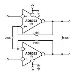
TPC 20. Multitone Power Ratio Test Circuit
