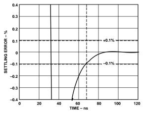
TPC 13. Settling Time to 0.1%,  $V_S = \pm 12 V$ , Step Size = 2 V p-p, G = +2,  $R_L = 500 \Omega$
