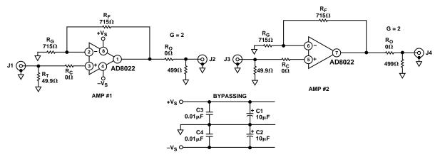
Figure 8. Evaluation Board Schematic
