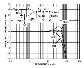
TPC 5. Frequency Response vs. Capacitive Load,  $C_L$  = 0 pF, 30 pF, and 50 pF,  $R_S$  = 0  $\Omega$
