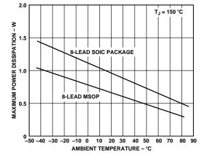
*Figure 2. Plot of Maximum Power Dissipation vs. Temperature*
