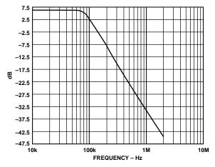
Figure 7. Frequency Response of Sallen-Key Filter
