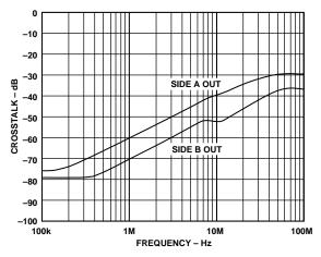
TPC 33. Output-to-Output Crosstalk vs. Frequency,  $V_S = \pm 2.5 V$
