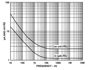
Figure 1. Current and Voltage Noise vs. Frequency
