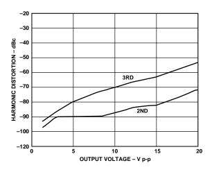
TPC 18. Distortion vs. Output Voltage,  $V_S = \pm 12$  V, G = +2, f = 1 MHz,  $R_L = 500 \Omega$ ,  $R_F = 715 \Omega$
