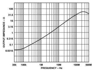
TPC 34. Output Impedance vs. Frequency,  $V_S = \pm 12 V$
