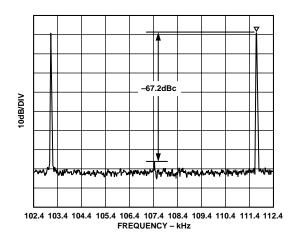
TPC 22. Multitone Power Ratio:  $V_S = \pm 12 V$ ,  $R_L = 500 \Omega$ , Full Rate ADSL (DMT), Upstream
