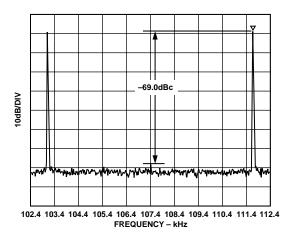
TPC 24. Multitone Power Ratio:  $V_S = \pm 6 V$ ,  $R_L = 500 \Omega$ , Full Rate ADSL (DMT), Upstream
