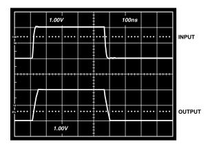
TPC 12. Noninverting Large Signal Pulse Response,  $R_L = 500 \ \Omega$ ,  $V_S = \pm 2.5V$ , G = +1,  $R_F = 0$
