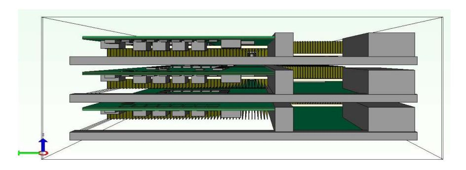
Model includes 2mm Rails on each side of the ATCA Blade Any other Air Flow Obstruction to Consider?
