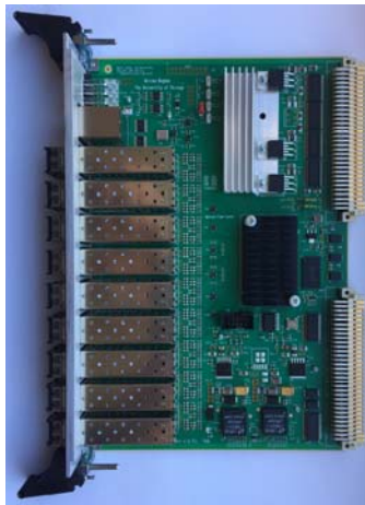
Figure 4. The Optical Fiber Center Module. This Double Width, 6U VME Module is fitted with 18 SFP Links running at max 6.2Gbps each.
