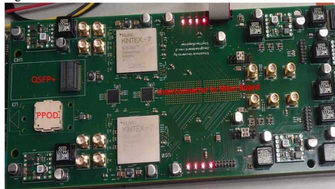
Fig. 7. The second prototype of the Daughter Board.
