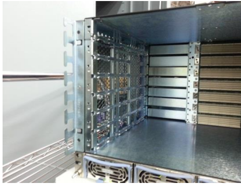
Figure 20: Cable Management Frame
