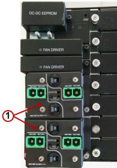
Figure 4: DC PEMs (all other components - see AC config)
