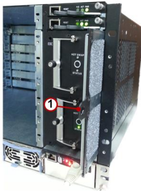
Figure 23: Air Filter Removal for Inspection
