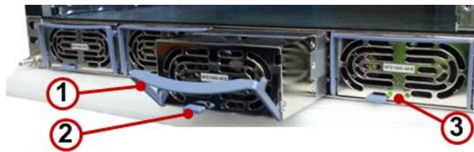
Figure 24: Power Supply Replacement-AC Configuration
