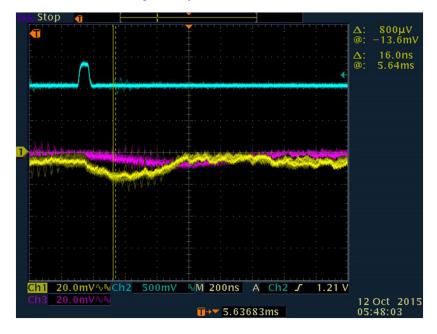
Channel 2 =L1A pulse Channels 1,3 = Voltage on test resistor Math(Ch1 - Ch3) =>  $I_{VCCINT}$  = 1.46A<sub>RMS</sub>
