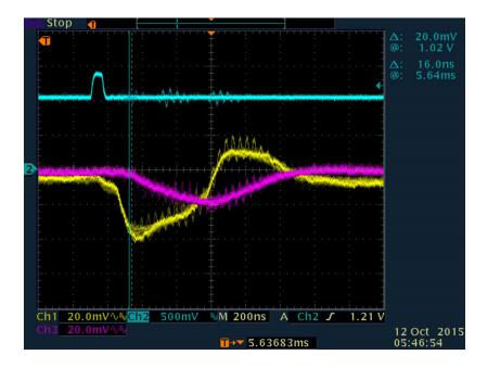
Channel 2 =L1A pulse Channels 1,3 = voltage on test resistor Math(Ch1 - Ch3) =>  $I_{VCCINT}$  = 1.463A<sub>RMS</sub>
