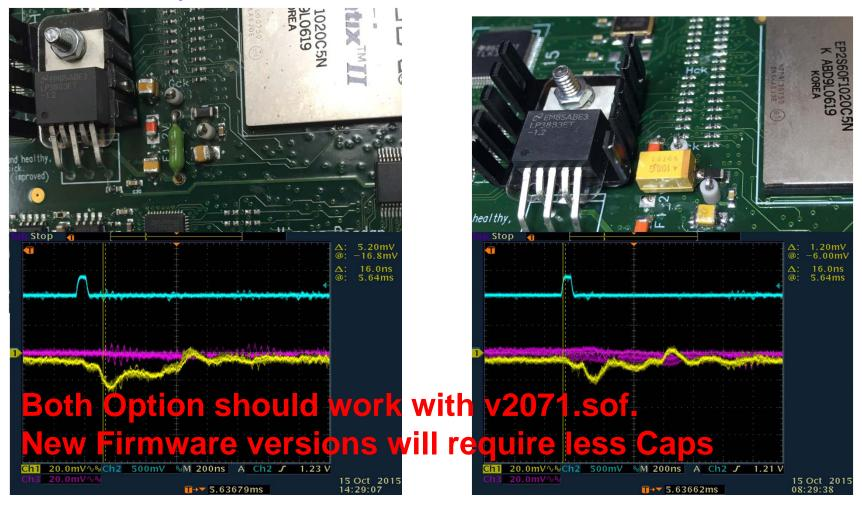
Replacing C26, C27 from 10uF to 470uF or larger shows improvement of VCCINT and +1.2V stability during the brief intervals of increased demand.
